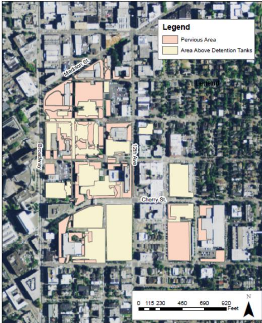
Figure 8: Map of the Seattle University campus with available treatment type data (2012) for run-off with the options of pervious area (including current rain gardens) and areas that feed cisterns.
