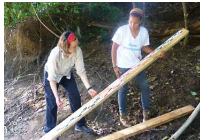
Josephine Archibald, faculty adviser for ENSC 17.2 and Maria Jose Corder Fernandez, a student from University of Central America, install stage gauges for collection of data on the Rio Ochomogo in Nicaragua.
